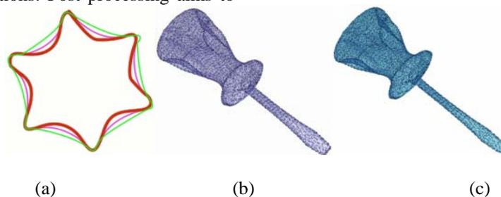
Figure 2. (a) Automatic intermediate slice generation. First slice is in red, second slice is in green and the intermediate slice is shown in purple. (b) Reconstructing the original object (c) Edited object
