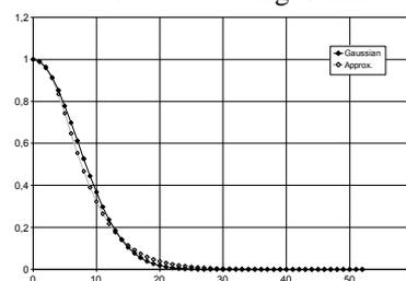
Figure 1. Gaussian  $\sigma=10$  and simulation using three exponential curves
