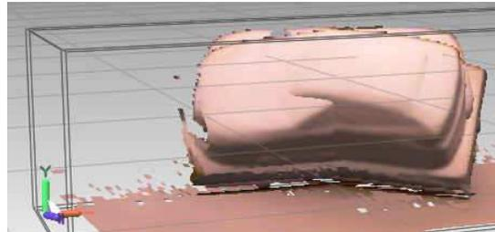
In the figure above, two overlapping scan views of a simple car model are shown. The number of points in  $A$  and  $B$  are 6107 and 6518, respectively. Using 16 steps over 40 degrees for the three rotation axes and 16 steps for the three translation directions over the bounding boxes of  $A$  and  $B$ ,  $I$  was computed  $16^6 = 16.8$  million times. The highest  $I$  produced the correct  $M$  and hence registration of the two scan views, found in a few minutes of computation time.
